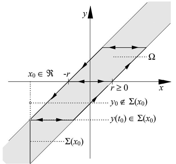
figure 6. Rate-independent characteristic of the play operator  $H_r$
