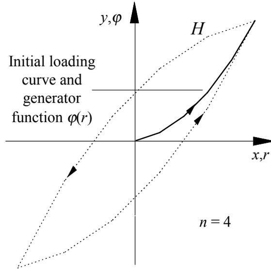
figure 7. Initial loading curve and generator function  $\varphi(r)$
