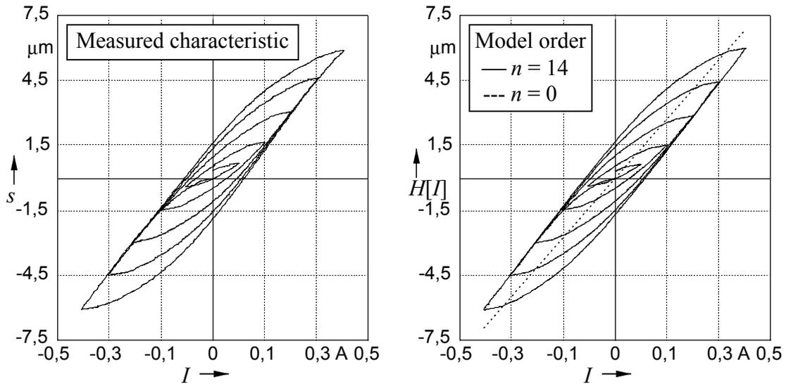
figure 11. Measured and modeled hysteretic displacement-current relation
